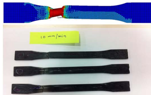
Fig. 10: Correlation of CAE and Test failure of specimen at 10mm/min strain rate.
