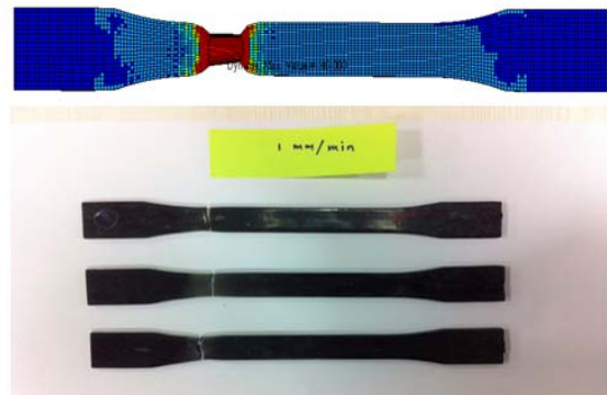
Fig. 9: Correlation of CAE and Test failure of specimen at 1mm/min strain rate.
