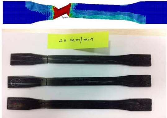
Fig. 11: Correlation of CAE and Test failure of specimen at 20mm/min strain rate.
