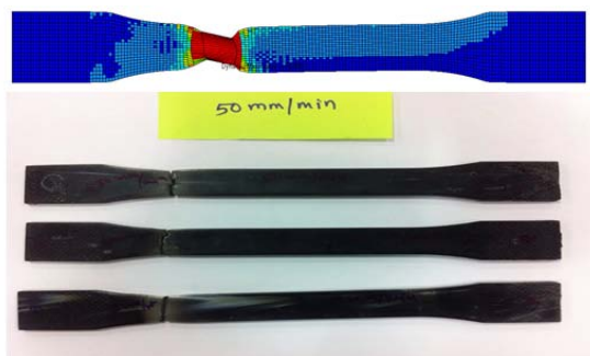
Fig. 12: Correlation of CAE and Test failure of specimen at 50mm/min strain rate.
